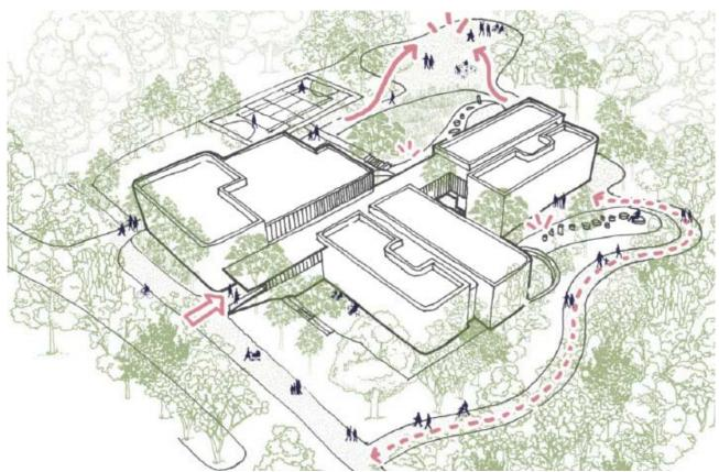
Figure 8: Illustration of massing. Build split into 3 distinct blocks with spinal connection route
